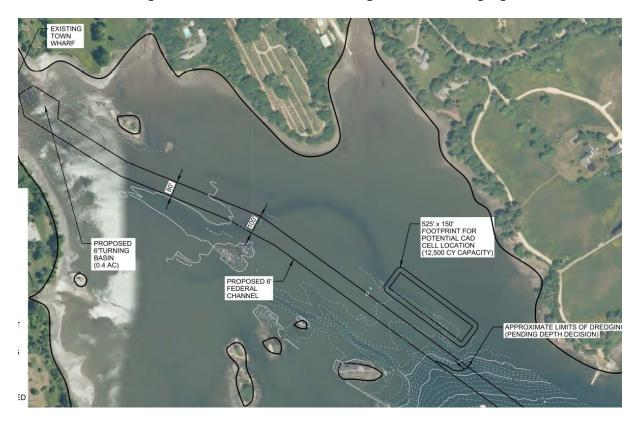
Figure E-4: New Channel Showing Limits of Dredging
